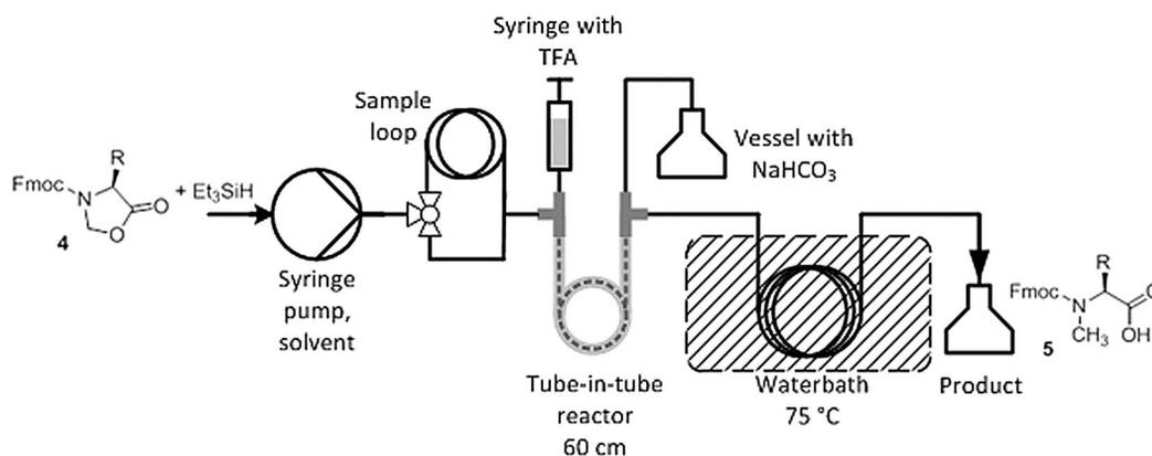
Figure 2. Flow reactor used for the second step of the NMA synthesis.
