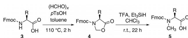
Scheme 1. *N*-Methylation of amino acids in two steps according to Freidinger et al. Fmoc = 9-fluorenylmethoxycarbonyl, TFA = trifluoroacetic acid.
