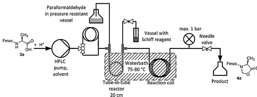
Figure 3. Flow tube-in-tube reactor used for the synthesis of Fmoc-oxazolidinones.
