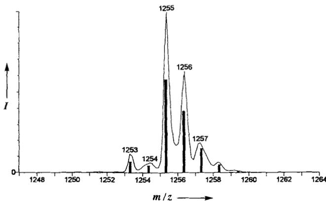
Fig. 1. Negative ionization electrospray mass spectrum of **1**. The calculated isotopic pattern for  $C_{26}H_{36}O_{11}Fe$  is indicated by the bars.
