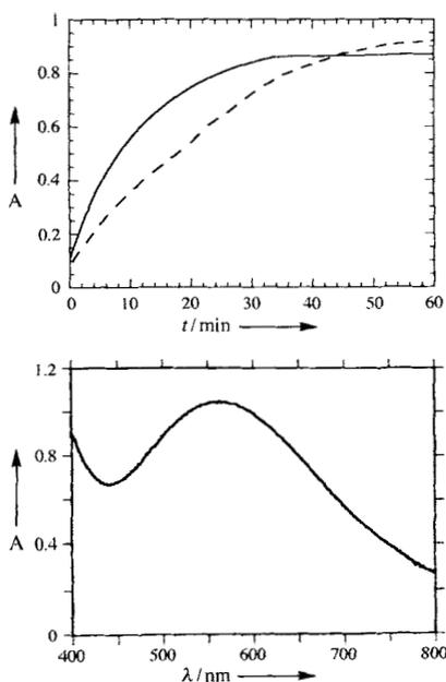
Fig. 2. Top: Absorbance at 560 nm versus time for the reaction of **1** [0.75 mM] with  $H_2O_2$  (3 equiv., —) or  $O_2$  (diffusing into the UV cell) and 15 equiv. of ascorbate (---). Bottom: UV/Vis spectrum recorded at the end of the reaction.
