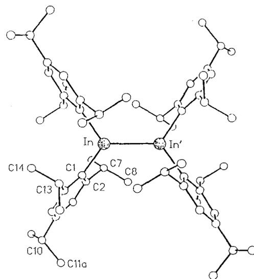
Fig. 1. Molecular structure of **1**. Selected bond lengths [ $\text{\AA}$ ] and angles [ $^\circ$ ]: In–In' 2.775(2), In–C1 2.184(7); In'–In–C1 121.6(2), C1–In–C1' 116.8(4).
