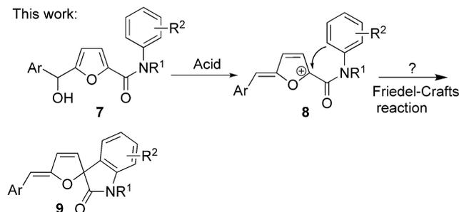
**Scheme 1.** Intramolecular trapping of the carbocation derived from a five-membered aromatic ring.
