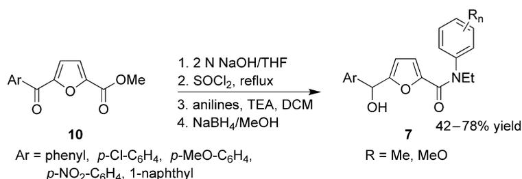
**Scheme 2.** Synthesis of precursors **7** for cyclization.
