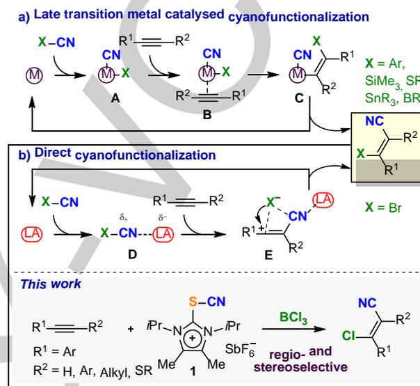
**Scheme 1.** Synthesis of substituted acrylonitriles from alkynes.
