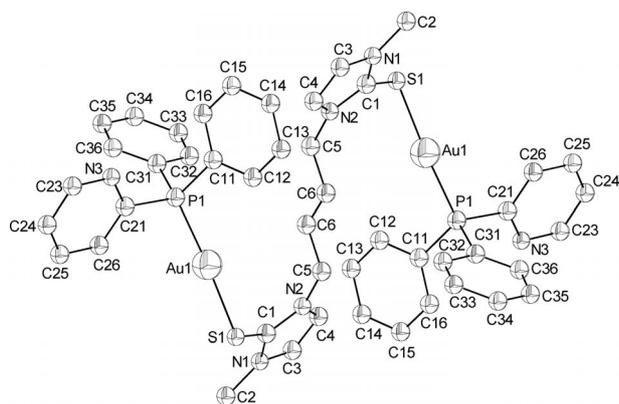
Figure 7. ORTEP representation at 50% probability and atom numbering scheme for the complex cation [Au<sub>2</sub>(PPh<sub>2</sub>py)<sub>2</sub>(Bbit)]<sup>2+</sup> in **13**. All hydrogen atoms, counter anions and solvents (CH<sub>2</sub>Cl<sub>2</sub>) are omitted for clarity. Selected bond lengths [Å] and angles (°): Au1–S1 2.313(2), S1–C1 1.726(9), Au1–P1 2.264(2), P1–Au1–S1 173.77(7), C1–S1–Au1 106.5(3), N1–C1–S1 124.4(8), N2–C1–S1 128.1(8).
