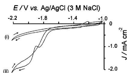
**Figure 1.** Cyclic voltammograms of scans at 5 mVs<sup>-1</sup> for an indium working electrode and a platinum mesh counter electrode versus Ag/AgCl (3 M NaCl) in [Emim][TFA] with i) Ar or ii) CO<sub>2</sub> atmospheres. Only the second consecutive cyclic voltammogram is shown for clarity.
