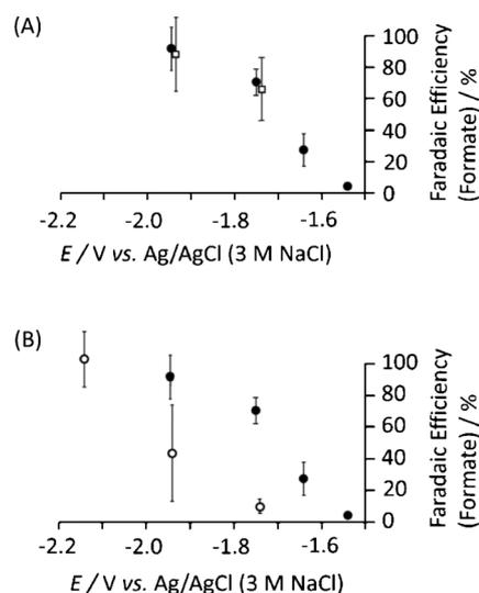
**Figure 6.** (A) Comparison of tin (open squares) and indium (closed circles) electrodes for the Faradaic efficiency of formate production from carbon dioxide in a matrix of 2 mL [Emim][TFA] + 1 mL D<sub>2</sub>O (pD 6.7) at various applied potentials. (B) Comparison of lead (open circles) and indium (closed circles) electrodes for the Faradaic efficiency of formate production from carbon dioxide in a matrix of 2 mL [Emim][TFA] + 1 mL D<sub>2</sub>O (pD 6.7) at various applied potentials.
