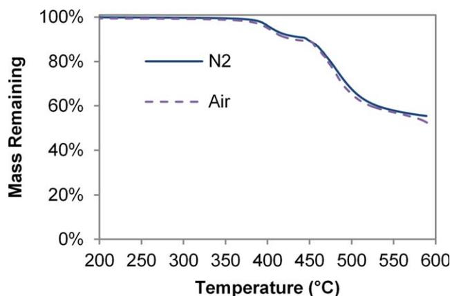
**FIGURE 12** TGA traces of cured SiCy-3 (**3**) in nitrogen and air. [Color figure can be viewed in the online issue, which is available at [wileyonlinelibrary.com](http://wileyonlinelibrary.com).]
