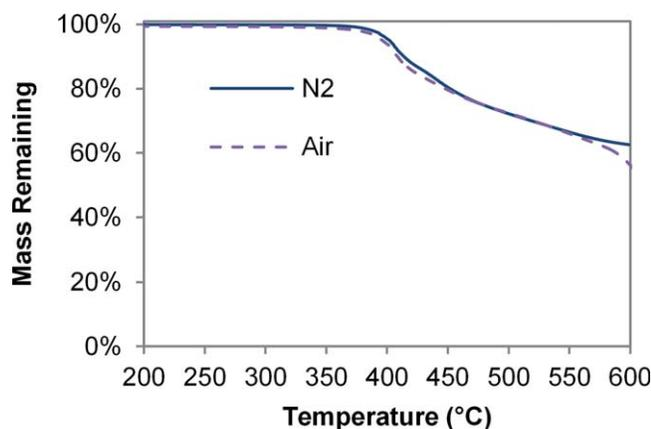
**FIGURE 13** TGA traces of cured SiCy-3 (**3**)/LECy (mixed in equal parts by weight before cure) in nitrogen and air. [Color figure can be viewed in the online issue, which is available at [wileyonlinelibrary.com](http://wileyonlinelibrary.com).]
