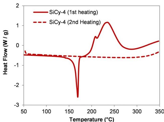
**FIGURE 5** Nonisothermal DSC of SiCy-4 (6). [Color figure can be viewed in the online issue, which is available at [wileyonlinelibrary.com](http://wileyonlinelibrary.com).]
