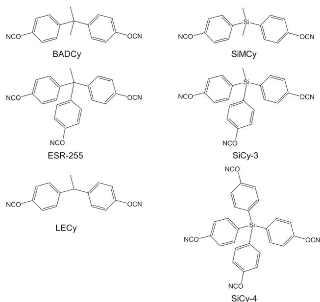
**FIGURE 3** Chemical structure of monomers utilized for comparative studies.
