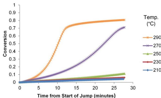
**FIGURE 6** Isothermal cure kinetics of SiCy-3 (3) after purification by flash chromatography. [Color figure can be viewed in the online issue, which is available at [wileyonlinelibrary.com](http://wileyonlinelibrary.com).]
