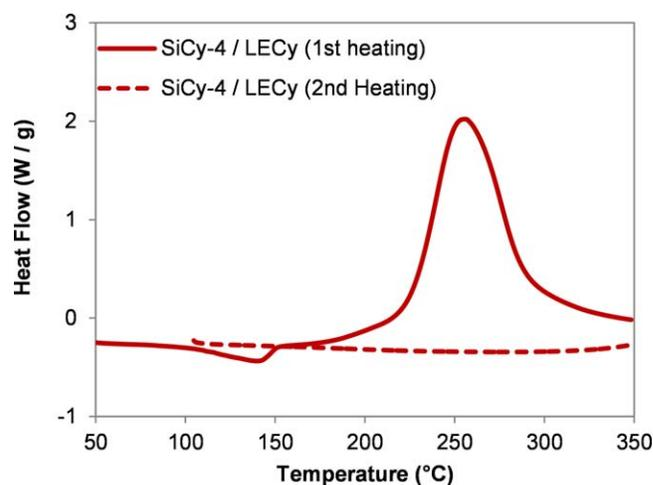
**FIGURE 9** Nonisothermal DSC of SiCy-4 (**6**) cocured with an equal weight of LECy. [Color figure can be viewed in the online issue, which is available at [wileyonlinelibrary.com](http://wileyonlinelibrary.com).]
