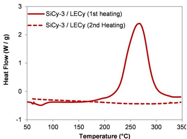
**FIGURE 8** Nonisothermal DSC of SiCy-3 (**3**) cocured with an equal weight of LECy. [Color figure can be viewed in the online issue, which is available at [wileyonlinelibrary.com](http://wileyonlinelibrary.com).]
