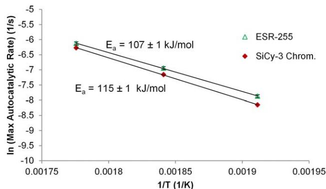
**FIGURE 7** Arrhenius plot showing maximum autocatalytic reaction rates of SiCy-3 (3, purified by chromatography) and ESR-255. [Color figure can be viewed in the online issue, which is available at [wileyonlinelibrary.com](http://wileyonlinelibrary.com).]
