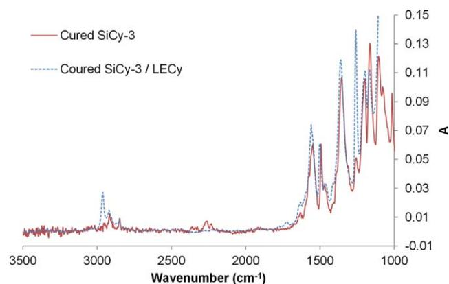
**FIGURE 10** FTIR spectra of SiCy-3 (**3**) and a mixture of equal parts SiCy-3 and LECy, after cure for 24 h at 210 °C. [Color figure can be viewed in the online issue, which is available at [wileyonlinelibrary.com](http://wileyonlinelibrary.com).]
