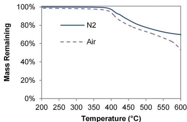
**FIGURE 14** TGA traces of cured SiCy-4 (**6**)/LECy (mixed in equal parts by weight before cure) in nitrogen and air. [Color figure can be viewed in the online issue, which is available at [wileyonlinelibrary.com](http://wileyonlinelibrary.com).]
