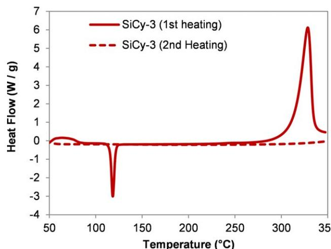
**FIGURE 4** Nonisothermal DSC of SiCy-3 (**3**). [Color figure can be viewed in the online issue, which is available at [wileyonlinelibrary.com](http://wileyonlinelibrary.com).]
