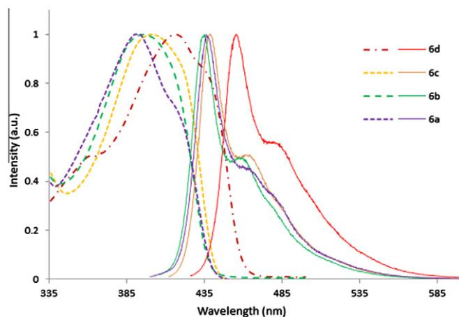
**Figure 2.** UV-vis and fluorescence spectra of tetramers **6a–d** in  $\text{CH}_2\text{Cl}_2$  solution. The dashed line represents the UV-vis spectrum and the solid line represents the fluorescence spectrum.
