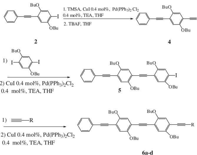
**Scheme 2.** Synthesis of phenylene-acetylene tetramers with various fluorescent chromophores.
