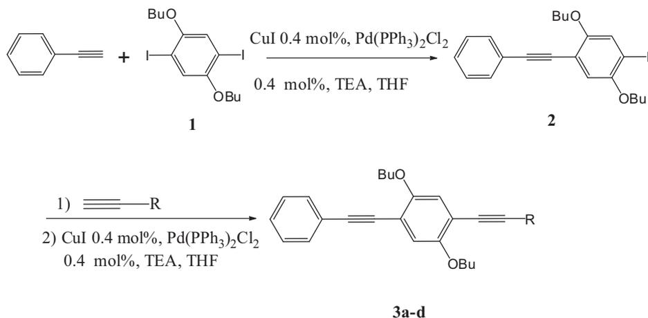
**Scheme 1.** Synthesis of phenylene-acetylene trimers with various fluorescent chromophores.
