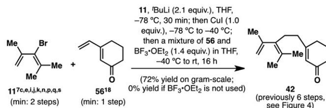
**Fig. 6.** A scalable 1,6-addition reaction resulting in a compound bearing both an A-ring precursor and a C-ring, which then became the focal point of this research project.
