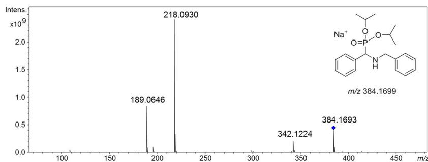
**Figure 2.** High-resolution ESI-FTICR tandem mass spectrum of  $[M+Na]^+$  ion of compound **1** at  $m/z$  384.1693.
