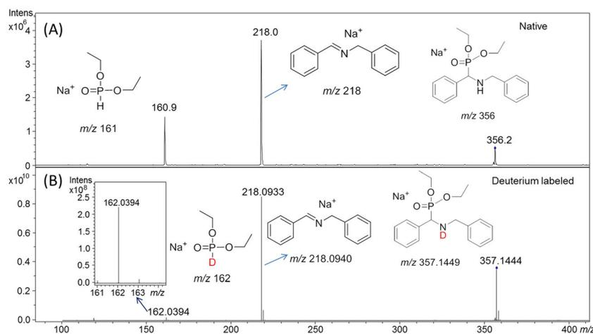
**Figure 3.** ESI tandem mass spectra of compound **2** in positive ion mode: (A) ESI-MS/MS of [M+Na]<sup>+</sup> ion at *m/z* 356 and (B) ESI-FT-ICR-MS/MS of deuterium-labeled [d-M+Na]<sup>+</sup> ion at *m/z* 357.1449.
