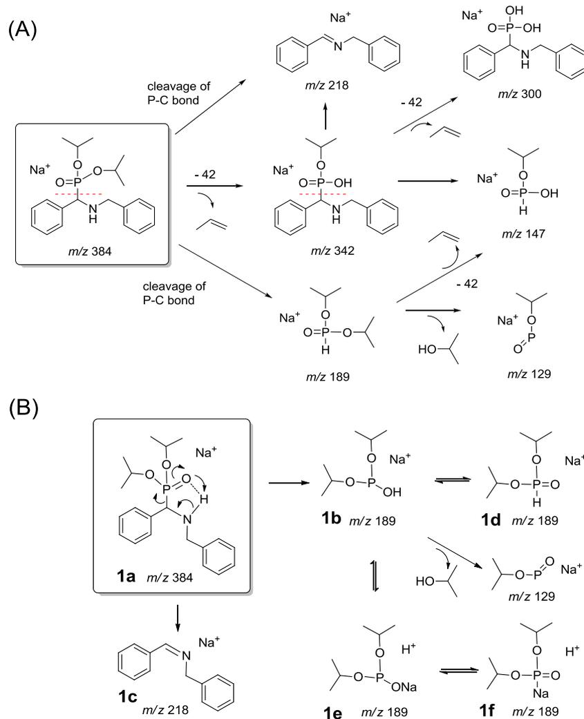
**Scheme 2.** (A) Possible fragmentation pathways of  $[M+Na]^+$  ion of compound **1**. (B) Proposed rearrangement mechanism for the intramolecular hydrogen migration.
