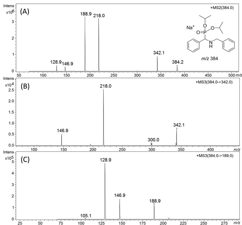
**Figure 1.** ESI tandem mass spectra of compound 1 in positive ion mode: (A) ESI-MS/MS of  $[\text{M}+\text{Na}]^+$  ion at  $m/z$  384; (B) ESI-MS<sup>3</sup> of product ion at  $m/z$  342; and (C) ESI-MS<sup>3</sup> of the rearrangement ion at  $m/z$  189.
