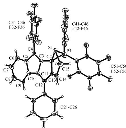
Figure 2. Molecular structure of compound **23** (thermal ellipsoids are shown with 30% probability). Selected bond lengths (Å) and angles (°): C2–B1 1.589(3), S1–B1 1.984(2), C2–S1 1.887(2), C2–C13 1.505(2), C13–C14 1.333(3), C14–C15 1.500(3), C2–C3 1.477(2), C3–C4 1.357(3), C3–C11 1.469(3), C11–C12 1.372(3), C11–C10 1.467(3), C12–C13 1.471(3), C3–C2–S1 128.5(1), C3–C2–B1 128.8(2), C4–C3–C2 142.7(2).
