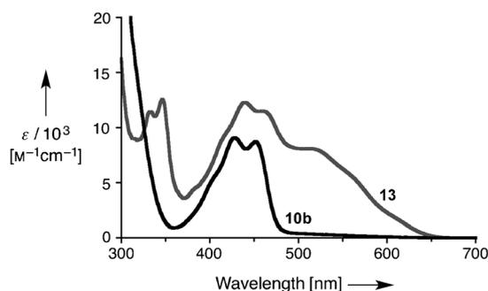
Figure 4. UV/Vis absorption spectra of **10b** (black) and **13** (gray) in acetonitrile.
