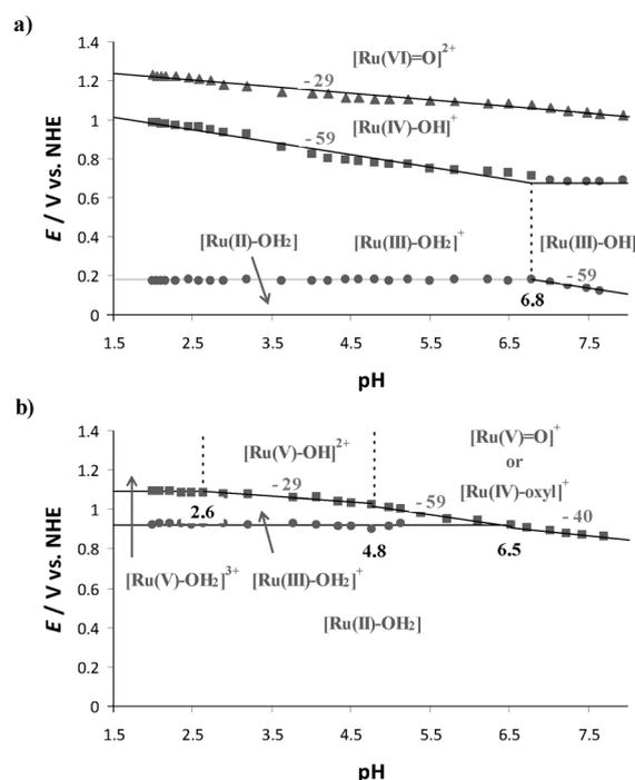
**Figure 4.** Pourbaix diagrams of a) complex **4** and b) complex **5**, in the range 1.5 < pH < 8.0 ( $pK_a$  values are denoted by the vertical dashed lines). Experimental conditions: Pourbaix diagrams of complexes **4** and **5** (30  $\mu$ M) were obtained from DPV measurements, in a 0.1 M Britton-Robinson buffer solutions in the range of 1.5 < pH < 8.0. The pH of the solution was changed by using a 0.2 M NaOH aqueous solution.
