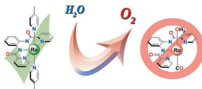
**No CO-operation:** Two single-site ruthenium complexes, based on a tetradentate ligand, despite structural similarities, display a remarkable difference in their catalytic and chemical behavior (see picture). The fact that the CO-containing complex is formed in the catalytic oxidation of water suggests a novel pathway for the deactivation of ruthenium-based catalysts.
