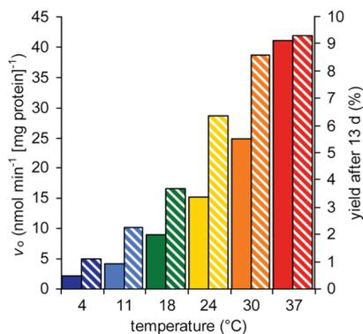
**Figure 4.** Dependence of initial rate ( $v_0$ , solid bars) and HPLC yield after 13 d (%), lined bars) on temperature for reaction of 3-methoxybenzyl alcohol **5** acceptor (89 mM) and  $\alpha$ -D-glucuronyl fluoride **2** donor (89 mM) (100 mM phosphate buffer, pH 7.5).
