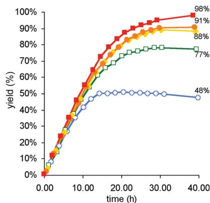
**Figure 6.** Reaction yield against time for reaction of CMO-DHEA **8** acceptor (1.4 mM) and varying equivalents of  $\alpha$ -D-glucuronyl fluoride **2** donor (100 mM phosphate buffer, pH 7.5, 37 °C). (blue circles, 1 equiv; green squares, 2 equiv; yellow diamonds, 3 equiv; orange circles, 4 equiv; red squares, 5 equiv).
