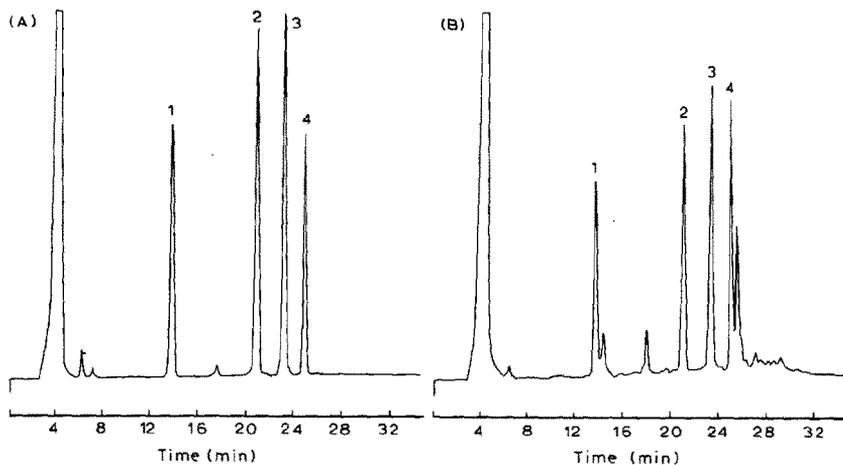
Fig. 1. Analytical h.p.l.c. separations of perbenzoylated carbohydrates: **1A**, standard mixture; **1B**, carbohydrate fractions of the acid-stage resin. Key: 1, mono-D-glucosylurea tetrabenzoate; 2, pentaerythritol tetrabenzoate; 3, D-glucose pentabenzoate; 4, di-D-glucosylurea octabenzoate. See Experimental for separation conditions.
