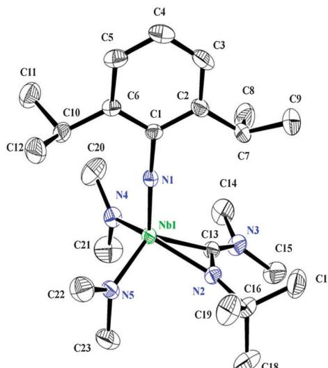
**Fig. 1** Thermal ellipsoids plot of **3** at 30% probability. Selected bonds ( $\text{\AA}$ ) and angles ( $^{\circ}$ ): Nb1–N1 1.783(2); Nb1–N2 2.128(2); Nb1–N4 2.005(2); N2–C13 1.292(3); N3–C13 1.341(3); N1–Nb1–N4 104.4(1); N4–Nb1–N5 104.7(1); Nb1–N1–C1 177.3(2).
