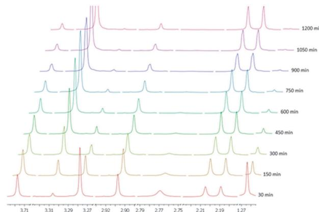
**Fig. 2** Evolution of the reaction of **3** with trisisopropylguanidine monitored by  $^1\text{H}$  NMR. Selected peaks are shown.
