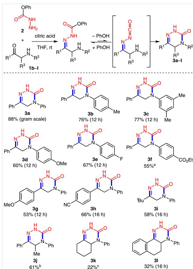
**Scheme 2** Scope of cascade reaction forming 1,2,4-triazin-3(2*H*)-ones. Reagents and conditions: phenyl carbazate (**2**, 1.0 equiv), **1b-1** (1.05 equiv), and citric acid (1.0 equiv) in THF (1.0 M) stirred at r.t. <sup>a</sup> Stirred at r.t. for 7 h, followed by reflux for 20 h. <sup>b</sup> Stirred at r.t. for 12 h, followed by reflux for 24 h. <sup>c</sup> Stirred at r.t. for 12 h, followed by reflux for 20 h.
