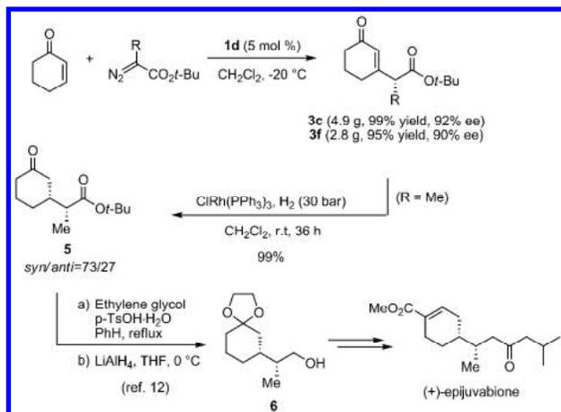
The feasibility of reducing catalyst loading and increasing reaction scale to a multi-gram scale was examined (Scheme 3). The loading of catalyst **1d** could be reduced to 5 mol% while maintaining excellent chemical yields and enantioselectivities.
