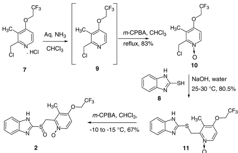
Figure 2. Synthesis of lansoprazole *N*-oxide.
