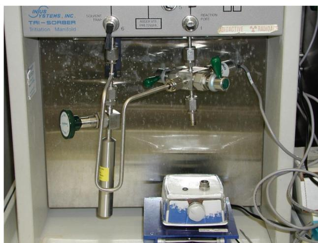
Figure 5. Tritiation manifold set-up used in labeling experiments.
