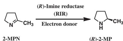
**Fig. 1.** Asymmetric Reduction of 2-MPN Using RIR in the Presence of an Electron Donor.
