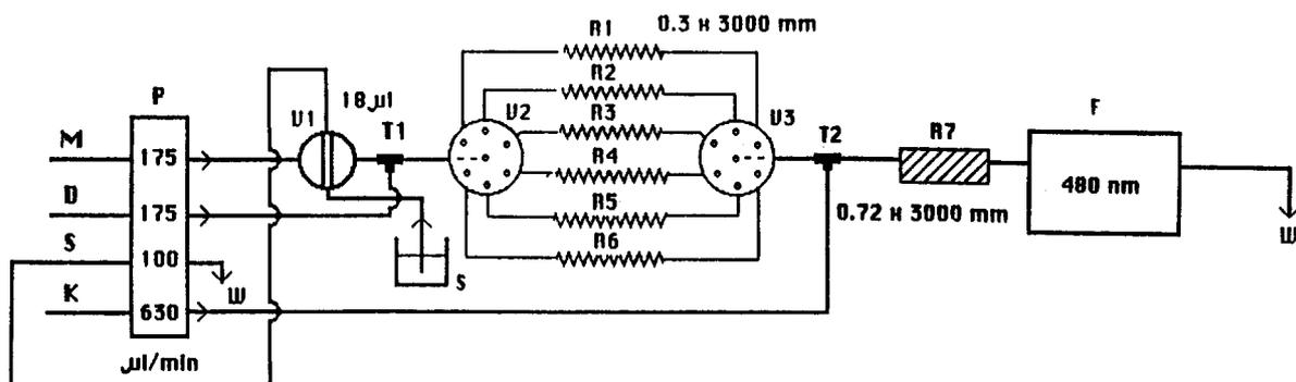
**Figure 2.** System schematic: P, peristaltic pump; M, methanol; D, DNPH reagent; S, sample; A, alkali reagent; W, waste; V1, sample injection valve; V2 and V3, simultaneously operated six-way selector valves connecting reactors R1–R6 individually at a time; T1 and T2, tees; R7, second-stage reactor; F, flow-through absorbance detector.
