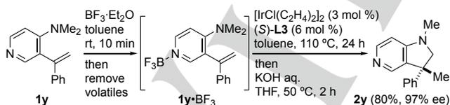
**Scheme 3.** Asymmetric Cycloisomerization of 4-(*N,N*-Dimethylamino)pyridine Derivative **1y**
