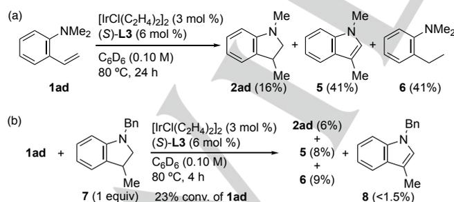
**Scheme 7.** Mechanistic Study Based on the Reaction of **1ad**
