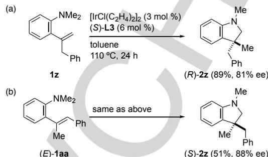
**Scheme 4.** Asymmetric Cycloisomerization of Potentially Interconvertible Alkenes **1z** and (*E*)-**1aa**
