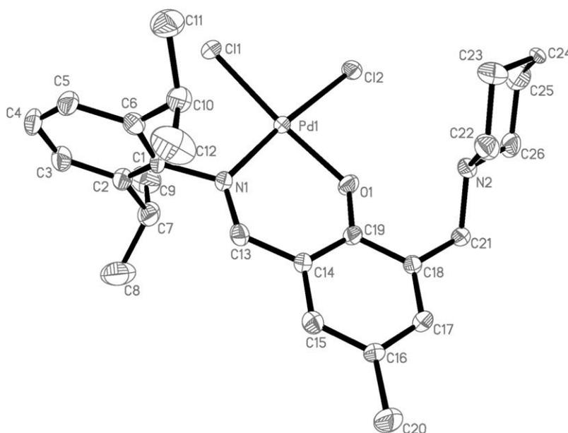
**Fig. 1.** Crystal structure of complex **2b**. Select bond lengths (Å) and angles (°): Pd1–Cl1 2.2939(8), Pd1–Cl2 2.3220(9), Pd1–N1 2.019(3), Pd1–O1 1.9687(19) and O1–Pd1–N1 91.03(11), O1–Pd1–Cl1 174.67(9), N1–Pd1–Cl1 94.28(8), O1–Pd1–Cl2 83.68(8), N2–Pd1–Cl2 174.66(8), Cl1–Pd1–Cl2 91.02(3).
