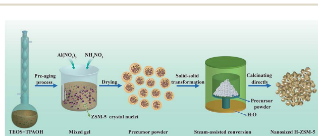
Fig. 1 Schematic diagram of centrifugation-free synthetic procedures for nanosized ZSM-5 with tunable Si/Al molar ratios.
