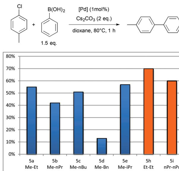
Fig. 5 Product yields in Suzuki–Miyaura cross-coupling of  $\text{PhB}(\text{OH})_2$  with  $p\text{-Cl-C}_6\text{H}_4\text{Me}$  using palladium complexes **5a–e** and **5h,i**. Reaction conditions:  $p\text{-tolyl chloride}$  (1 mmol), phenylboronic acid (1.5 mmol),  $\text{Cs}_2\text{CO}_3$  (2 mmol),  $[\text{Pd}]$  (1 mol%), dioxane (3 mL). Yields were determined by  $^1\text{H}$  NMR.
