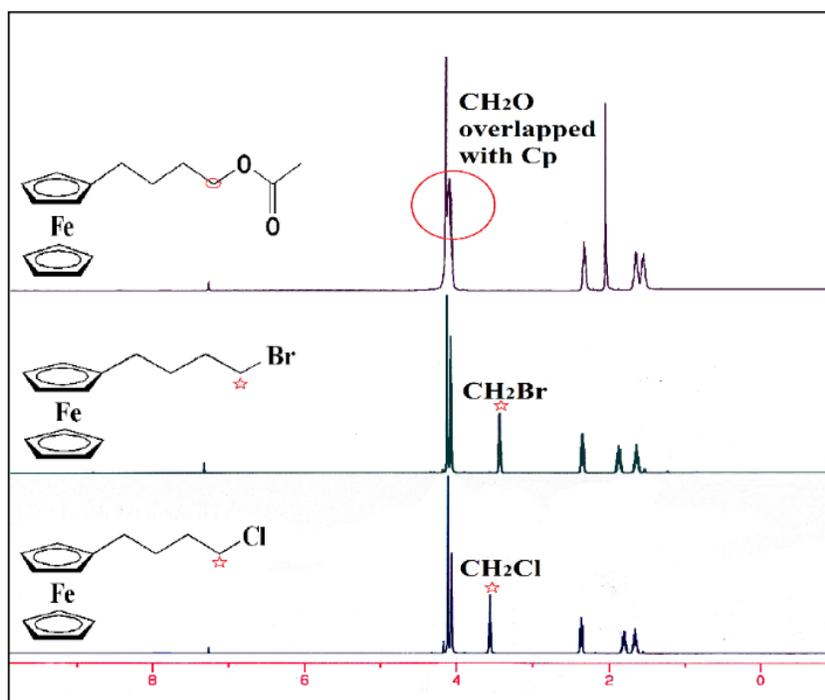
**Figure 3.** <sup>1</sup>H NMR spectra of 4-halobutylferrocenes **8a** and **8b** and 4-ferrocenylbutyl acetate **9**.
