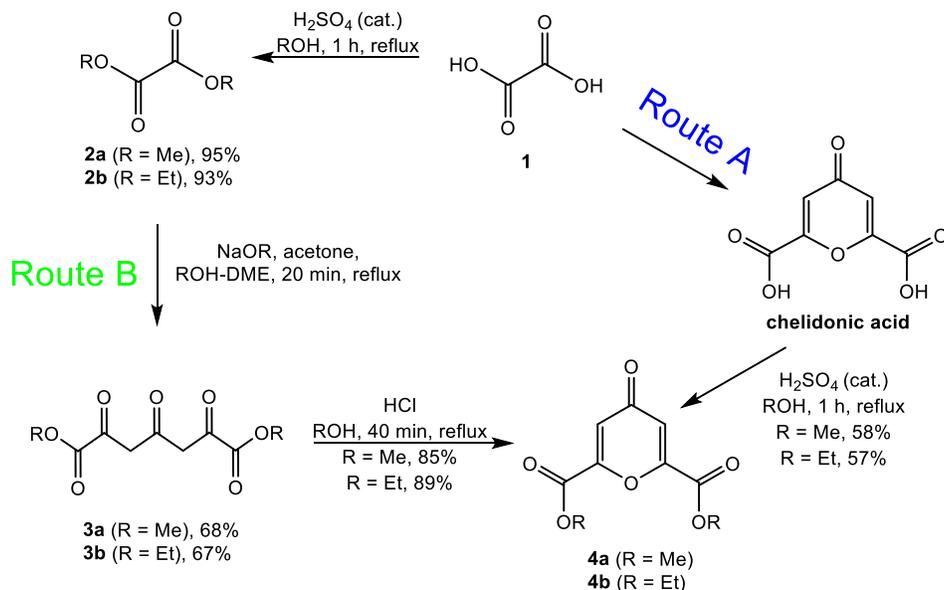
**Scheme 1.** Synthesis of dialkyl 4-oxo-4H-pyran-2,6-carboxylates **4** via the traditional method (Route A);<sup>24</sup> and via the modified procedure (Route B).<sup>25</sup>
