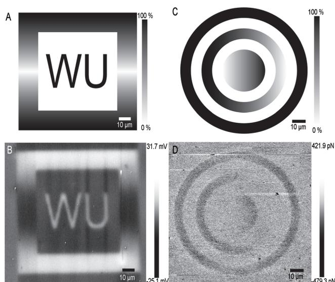
**Figure 1.** A and C) 8-bit images patterned by direct-write lithography (the scale bar is relative to the laser intensity). B) The resulting KFM image after deprotection. D) The adhesion channel for our patterned surface using PeakForce QNM.
