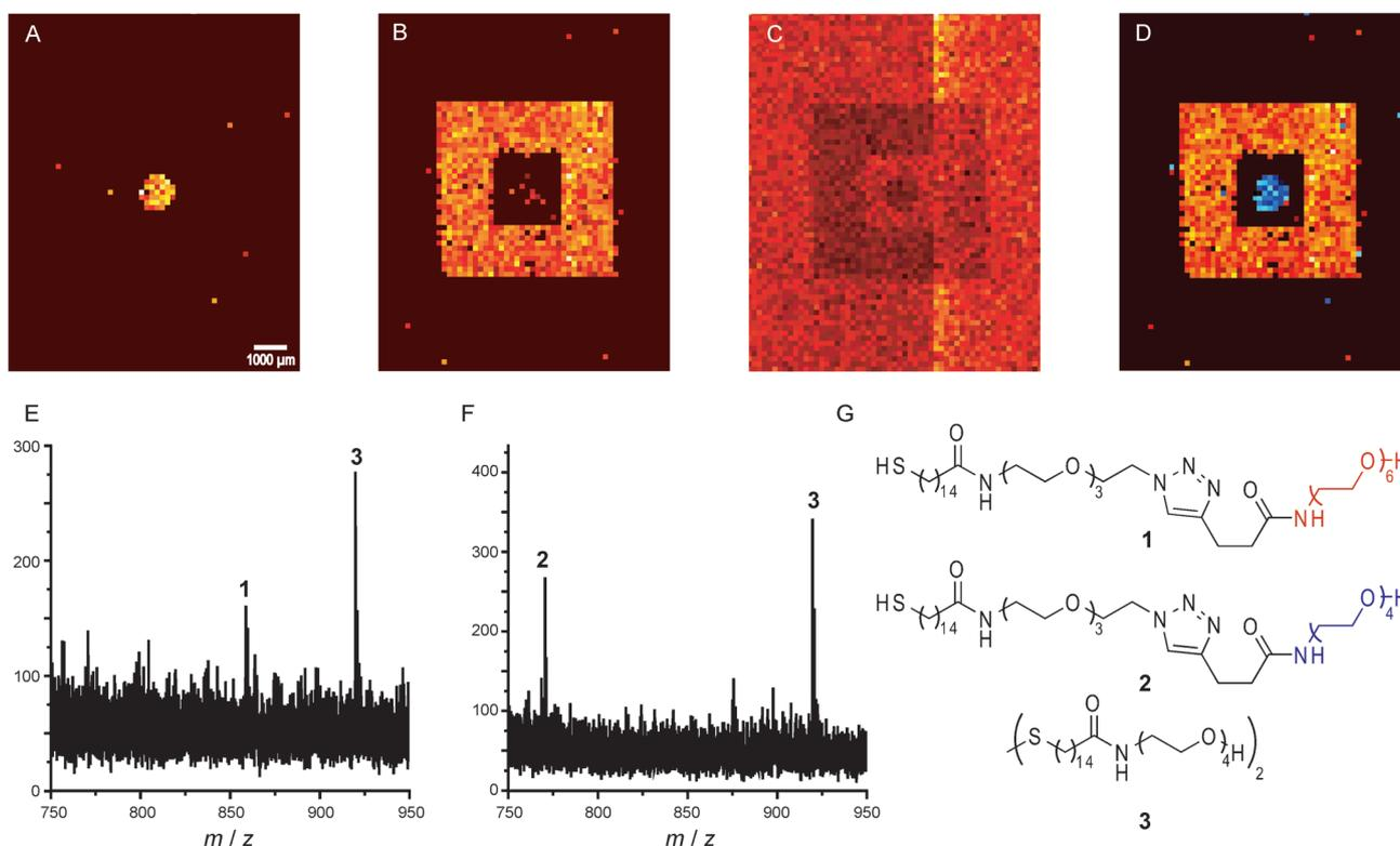
**Figure 2.** A,B,C) Heat maps generated after analysis for molecules **1**, **2**, and glycol-terminated photoprotected carboxylic acid monomer, respectively. D) Overlay of A and B. E,F) Representative MALDI-TOF spectrums for the circle and frame region, respectively. G) Molecules analyzed in the MALDI-TOF spectrum.
