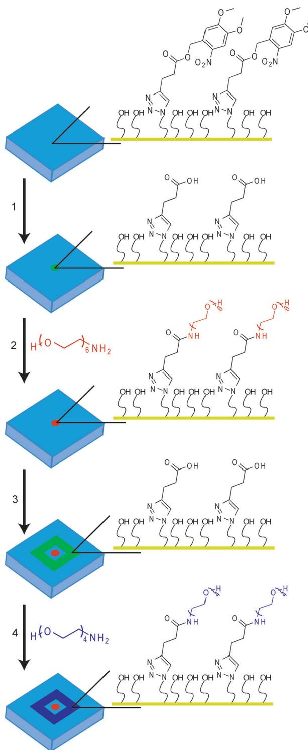
**Scheme 2.** Two-molecule patterning scheme. 1) Pattern circle, 2) activate carboxylic acid with EDC/HOAt and couple hexaethylene glycol amine, 3) pattern frame around the circle, and 4) activate carboxylic acid with EDC/HOAt and couple tetraethylene glycol amine.
