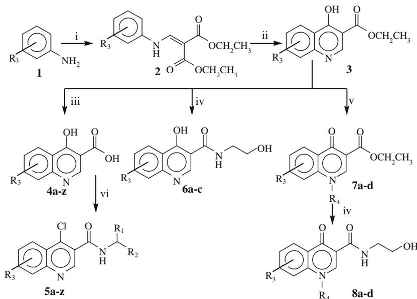
**Scheme 1.** Synthesis of quinoline derivatives. Reagents and conditions: (i) EMME, 3 h, rt, 130 °C; (ii) diphenyl ether, 2 h, rt, 250 °C; (iii) 1 M NaOH, 2 h, reflux; acetic acid was added until pH 2–3; (iv) ethanolamine, 2 h, rt, 170 °C; (v) R<sub>4</sub>I, DMF, 18 h, 60 °C; (vi) SOCl<sub>2</sub>, CHCl<sub>3</sub>, 4 h, rt, reflux; evaporate; NHR<sub>1</sub>R<sub>2</sub> was added.
