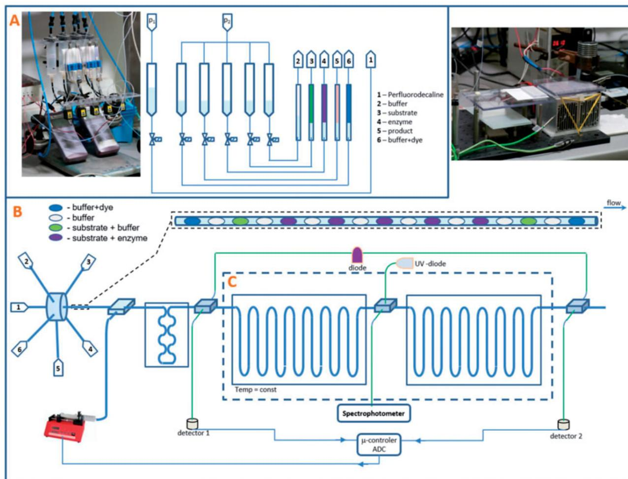
**Figure 1.** Scheme of experimental setup for determining the kinetic parameters of the enzymatic reaction: (A) reagent dosing system, (B) droplet generation system, and (C) reactor and detection system.
