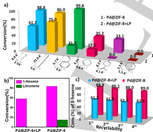
**Figure 3.** a) Hydrogenation of different substrates over Pd@ZIF-8 and Pd@ZIF-8+LP catalysts, b) Hydrogenation of mixed 1-hexene and limonene substrates catalyzed by Pd@ZIF-8 and Pd@ZIF-8+LP catalysts, and c) Recyclability test in the hydrogenation of 1-hexene over Pd@ZIF-8 and Pd@ZIF-8+LP catalysts.
