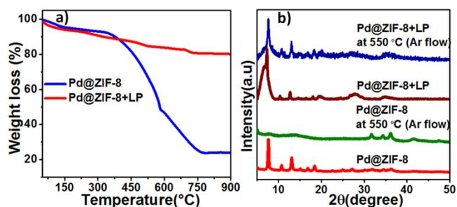
**Figure 2.** a) TGA of Pd@ZIF-8 (blue) and Pd@ZIF-8+LP xerogel (red), b) PXRD of Pd@ZIF-8 (red) and Pd@ZIF-8+LP xerogel (maroon) and their calcined products. Conditions: Calcinated at 550 °C under Ar for 1h.
