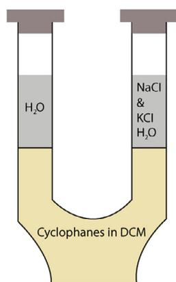
**FIGURE 2** Apparatus used for ion transport study [Color figure can be viewed at [wileyonlinelibrary.com](http://wileyonlinelibrary.com)]
