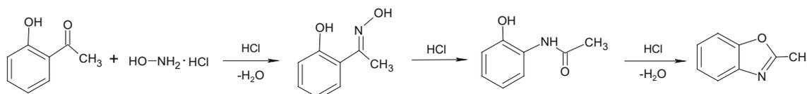
**Scheme 2** Steps observed in the direct-amidation–dehydrocyclization of 2-hydroxyacetophenone
