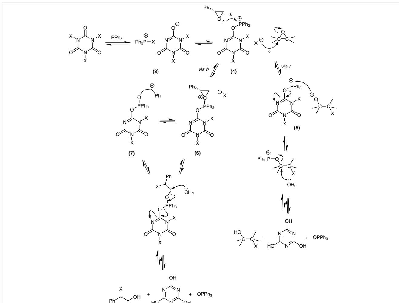
**Scheme 1** Mechanistic scheme for the formation of halohydrins from epoxides and TXCA/PPh<sub>3</sub>
