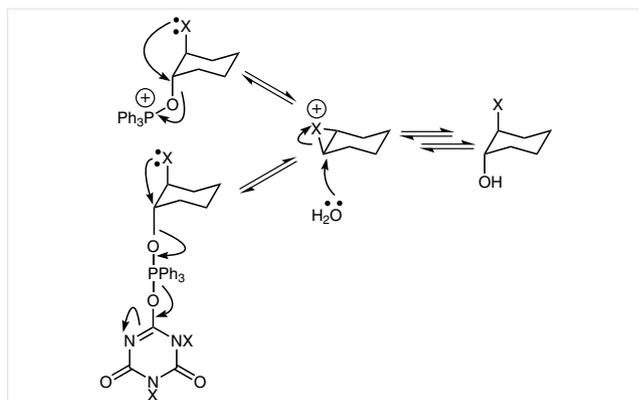
**Scheme 2** Mechanistic scheme for the formation of *trans*-halohydrins
