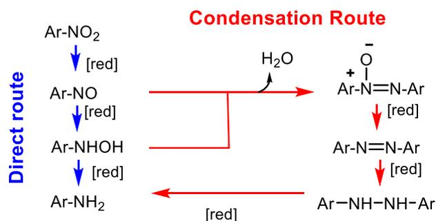
**Figure 1.** Proposed mechanism of nitrobenzene reduction.<sup>[25]</sup>
