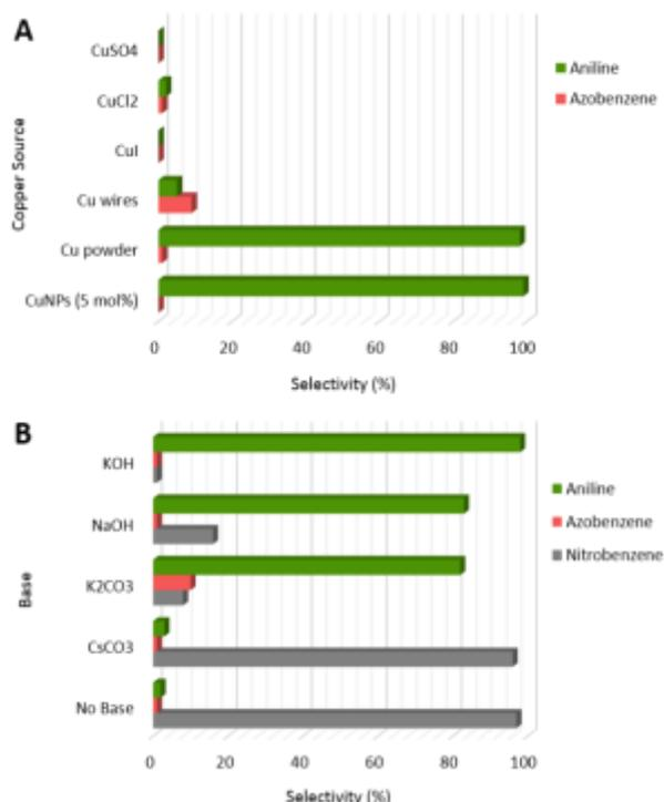
**Figure 2.** Influence of different copper sources (A) and bases (B) in the nitrobenzene TH. Reaction conditions: nitrobenzene (1 mmol), base (2 mmol), glycerol (40 mmol), Cu source (2 mmol), 130 °C, 5h.
