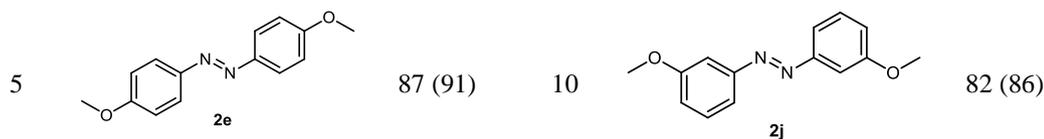
a) Reaction conditions: nitroarene (3mmol), Ethanolamine (20 mL), KOH (6 mmol), Cu NPs (5 mol%), T:55°C. b) Isolated yield. Reaction performed under conventional stirring in oil bath at 55 °C, 25 h. c) Isolated yield. Reaction performed under combined US (20.3 kHz, 15 Wcm<sup>-2</sup>) and MW (2.45 GHz, 15 W) irradiation (MW/US), 55 °C 1 h. Compound purity proved by <sup>1</sup>H-NMR and <sup>13</sup>C-NMR (see Supporting Info).
