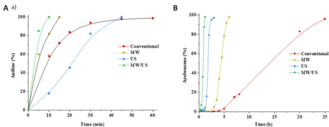
**Figure 5.** TH kinetic data of nitrobenzene catalysed by Cu NPs. (A) Glycerol, T: 130 °C and (B) Ethanolamine, T: 55 °C. Reaction conditions: nitrobenzene (1mmol), solvent (40 mmol), KOH (2 mmol), Cu NPs (5 mol%, <sup>a</sup>) when the reaction was performed under US/MW irradiation the catalyst was used in 2.5 mol %). Determined by GC-MS.
