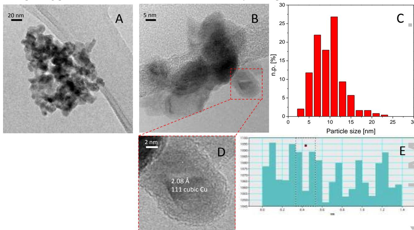
**Figure 3.** a) TEM, b) HR-TEM images and c)  $\text{Cu}$  particle size distributions of the  $\text{Cu}$  NPs catalyst prepared with glycerol as capping agent. d) detail of b) and e) measure of the spacing between the diffraction fringes observed in the zone highlighted by the red dashed square in b). Instrumental magnification: 50000 $\times$  and 300000 $\times$ , respectively. n.p.[%]= number of counted particles of diameter  $d_i$ .
