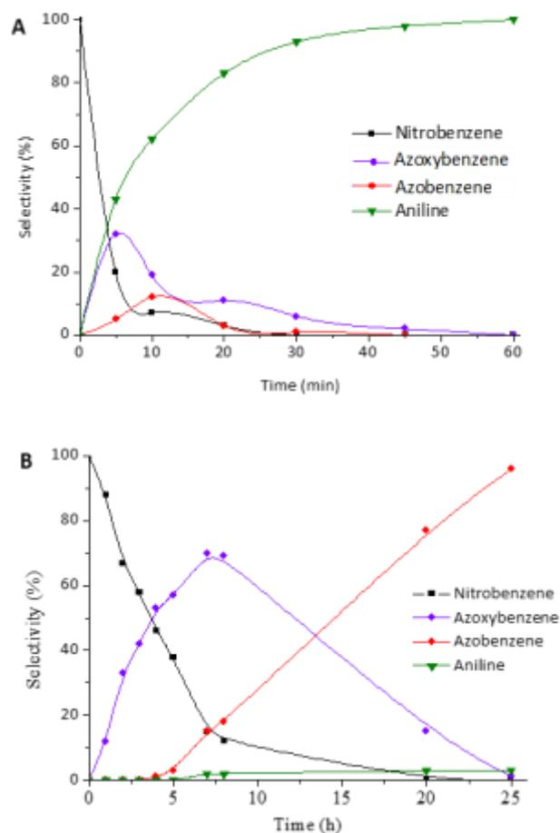
**Figure 4.** TH kinetics of nitrobenzene (A) Glycerol, T: 130 °C and (B) Ethanolamine, T: 55 °C. Reaction conditions: nitrobenzene (1 mmol), KOH (2 mmol), solvent (40 mmol), Cu NPs (5 mol%). Determined by GC-MS.
