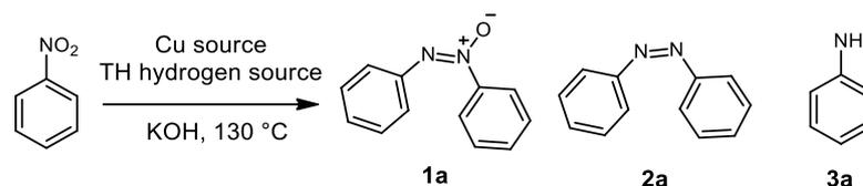
**Scheme 1.** Catalytic reduction of nitrobenzene to azoxy-, azobenzene, aniline.
