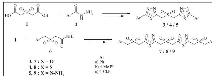
A new class of bis(oxadiazolyl/thiadiazolyl/triazolylmethyl)sulfones were prepared by the cyclocondensation of sulfonyldiacetic acid with aryl acid hydrazide and arylmethanesulfonylacetic acid hydrazide.
