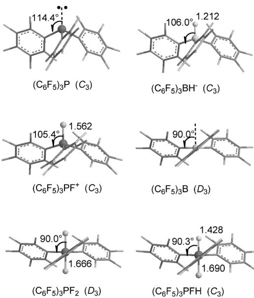
**Figure 2.** Optimised geometries of some P- and B-containing Lewis acids and bases. Bond lengths are given in Å angles in degrees.
