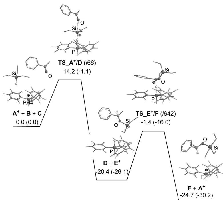
**Figure 3.** Reaction pathway for the hydrosilylation of ketones catalysed by **A**<sup>+</sup>. Relative free energies were calculated using B2PLYP-D3 and are given in kcal mol<sup>-1</sup>; enthalpies given in parentheses. Hydrogen atoms on substituents are omitted for clarity.
