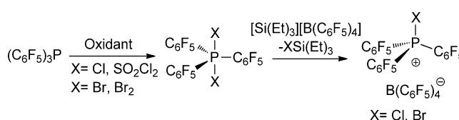
**Scheme 3.** Preparation of  $[(\text{C}_6\text{F}_5)_3\text{PCl}][\text{B}(\text{C}_6\text{F}_5)_4]$  and  $[(\text{C}_6\text{F}_5)_3\text{PBr}][\text{B}(\text{C}_6\text{F}_5)_4]$ .
