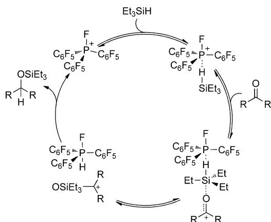
Scheme 4. Proposed mechanism for hydrosilylation catalysis by  $[(\text{C}_6\text{F}_5)_3\text{PF}]^+$ .
