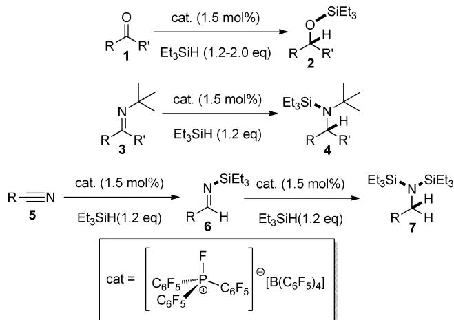
**Scheme 1.**  $[(C_6F_5)_3PF][B(C_6F_5)_4]$ -catalysed hydrosilylation of ketones (**1**), imines (**3**), and nitriles (**5**) to silyl enol ethers (**2**), *N*-silylamines (**4**), and *N*-silylimines (**6**) or *N,N*-disilylamines (**7**), respectively.
