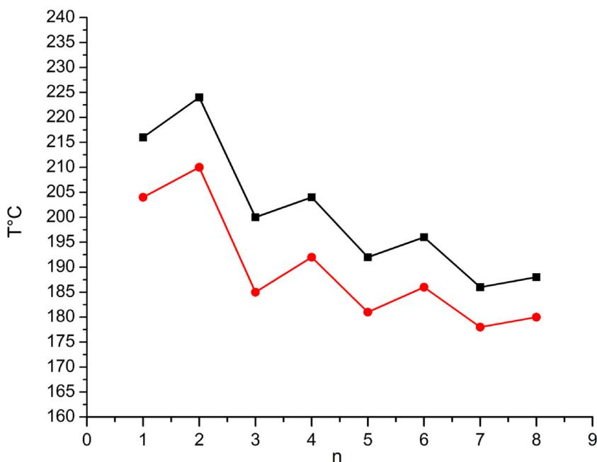
**Figure 3.** Clearing temperature ( $T_c$ ) as a function of alkyl chain length for 1,3,4-thiadiazoles series (black line) and silver(I) complexes series (red line).
