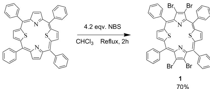
**Scheme 1.** Synthetic scheme for  $\beta$ -pyrrole substituted 21,23-dithiaporphyrin **1**.
