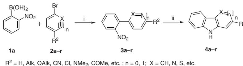
**Scheme 1** Synthesis of 2-substituted carbazoles and other indolo-fused systems. (i) Suzuki–Miyaura cross-coupling; (ii) Cadogan reductive cyclization.
