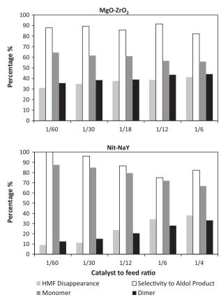
**Fig. 9.** Effect of catalyst to feed ratio by weight on the HMF disappearance, the selectivity to aldol products and the product distribution over MgO–ZrO<sub>2</sub> and Nit-NaY. Reaction conditions: temperature: 120 °C; reaction time: 16 h; total organics in solvent: 5 wt.%, HMF/acetone = 1 by moles; solvent: methanol/water = 1 by volume.
