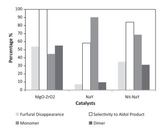
**Fig. 6.** Furfural disappearance, selectivity to aldol products, and product distribution for aldol condensation of furfural with acetone over MgO–ZrO<sub>2</sub>, NaY and Nit-NaY. Reaction conditions: temperature: 120 °C; pressure: 750 psig of helium; reaction time: 24 h; total organic in solvent: 5 wt.%; furfural:acetone = 1 by moles; catalyst: 15 mg; solvent: water/methanol = 1 by volume.
