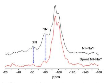
**Fig. 5.** <sup>29</sup>Si MAS NMR over the fresh and spent Nit-NaY catalyst. The spent Nit-NaY after two runs of furfural condensation with acetone at  $120 \degree$ C for 75 h lost 90% of nitrogen in zeolite framework.
