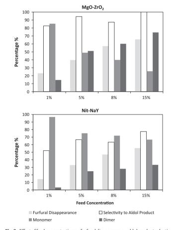
**Fig. 8.** Effect of feed concentration on furfural disappearance, aldol product selectivity and the product distribution over MgO–ZrO<sub>2</sub> and Nit-NaY. Reaction conditions: temperature: 120 °C; reaction time: 24 h; total organics/catalyst ratio of 6, furfural/acetone = 1 by moles; solvent: water/methanol = 1 by volume.
