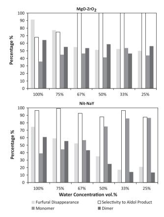
**Fig. 7.** Solvent effect on furfural disappearance and the product distribution over MgO-ZrO<sub>2</sub> and Nit-NaY. Reaction conditions: temperature: 120 °C; reaction time: 24h; total organic in solvent: 5 wt.%, furfural/acetone = 1 by molar; catalyst: 1/6 total organics by weight (15 mg); solvent: variation of methanol to water volumetric ratios.
