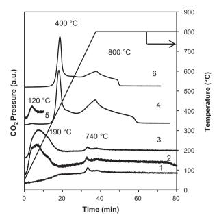
**Fig. 3.** CO<sub>2</sub> TPD-MS profiles over the fresh and spent MgO–ZrO<sub>2</sub> catalyst. Key: 1. Fresh MgO–ZrO<sub>2</sub>, background control experiment; 2. Fresh MgO–ZrO<sub>2</sub>; 3. Spent MgO–ZrO<sub>2</sub> calcined at  $600^{\circ}$ C for 1 h; 4. Spent MgO–ZrO<sub>2</sub>; 5. Spent MgO–ZrO<sub>2</sub>, signal at low temperature; 6. Spent MgO–ZrO<sub>2</sub>, background control experiment. The signals in Spectra 1, 2, 3 and 5 were multiplied by ten.
