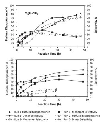
**Fig. 10.** TOS furfural disappearance and the selectivities to monomer and dimer over MgO–ZrO<sub>2</sub> and Nit-NaY. The second run was conducted by using the catalyst recycled from the first run. Reaction conditions: reaction volume: 75 mL; temperature:  $120^{\circ}$ C; pressure: 750 psig of helium; total organics 5 wt.%, furfural/acetone = 1 by moles; solvent: methanol/water = 2; catalysts: 250 mg, about 1/12 total organics by weight.
