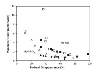
**Fig. 11.** Furfural disappearance as a function of molar ratio of furfural acetone monomer over dimer. The data are compared at methanol/water solvent volumetric ratio of 1 (solid symbols) and methanol/water volumetric ratio of 2 (open symbols).
