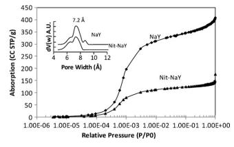
**Fig. 2.** The high resolution Ar adsorption isotherms and the pore size distribution of NaY and Nit-NaY. The results indicate that the Nit-NaY catalyst maintains pore size distribution and part of the crystal structure with the loss of pore volume and surface area to a degree. The unit of dV(w) is cm<sup>3</sup>/Å/g.
