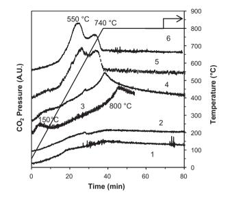
**Fig. 4.** CO<sub>2</sub> TPD-MS profiles over NaY, Nit-NaY and spent Nit-NaY. Key: 1. Fresh Nit-NaY, background control experiment; 2. Fresh NaY, background control experiment; 3. Fresh Nit-NaY; 4. Fresh NaY; 5. Spent Nit-NaY; 6. Spent Nit-NaY, background control experiment.
