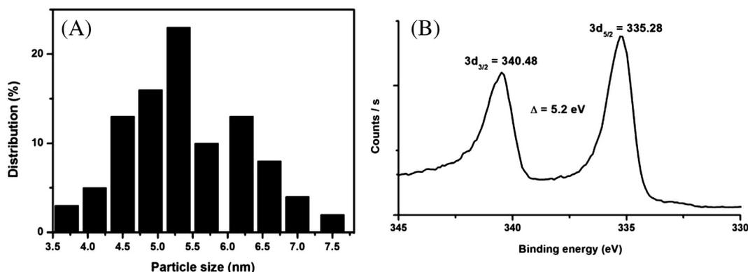
Fig. 2. Size histogram (A) and XPS spectrum (B) of supported Pd nanoparticles.
