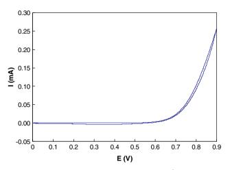
**Figure 1.** Cyclic voltammetry recorded at  $0.05 \text{ V s}^{-1}$  over a glassycarbon electrode (1 cm<sup>2</sup>) of a solution containing glycerol (0.05 M) and TEMPO ( $7.5 \times 10^{-3}$  M) in the presence of 0.2 M NaHCO<sub>3</sub>.
