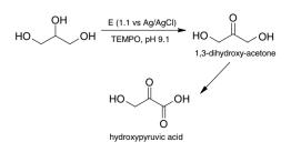
Scheme 2. Electrochemical oxidation of glycerol mediated by TEMPO in water affords DHA and, after longer reaction times, HPA.
