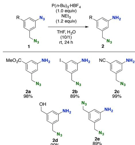
Figure 4. Aromatic azido-selective reduction of di- and triazides **1**.
