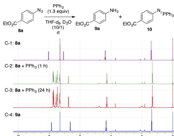
**Figure 2.** Monitoring the reaction between azide **8a** and triphenylphosphine in THF-*d*<sub>8</sub> and D<sub>2</sub>O (10/1, v/v) at room temperature by <sup>1</sup>H NMR.
