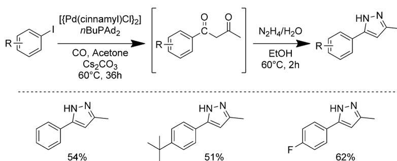
Scheme 2. One-pot synthesis of pyrazoles by (carbonylative)  $\alpha$ -arylation of ketones. 1) aryl iodide (1 mmol), acetone (2 mL),  $[\text{Pd}(\text{cinnamyl})\text{Cl}]_2$  (1 mol %),  $n\text{BuPAd}_2$  (4 mol %),  $\text{Cs}_2\text{CO}_3$  (2 mmol), CO (3 bar), 60°C, 36 h; 2)  $\text{N}_2\text{H}_4$  (6 mmol), EtOH (0.5 mL), 60°C, 2 h. Yields of the isolated products.
