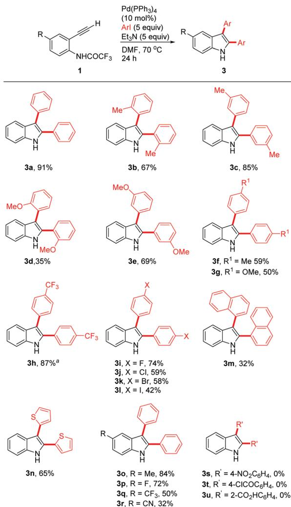
**Scheme 2** Substrate scope of *o*-ethynyltrifluoroacetanilides **1** and aryl iodides **2**. **1** (0.47 mmol, 1.0 equiv.), **2** (5.0 equiv.), Et<sub>3</sub>N (5.0 equiv.), Pd(PPh<sub>3</sub>)<sub>4</sub> (10 mol %) and DMF (3.0 mL), under N<sub>2</sub>, 24 h, isolated yields. <sup>a</sup> Reacted for 48 h.
