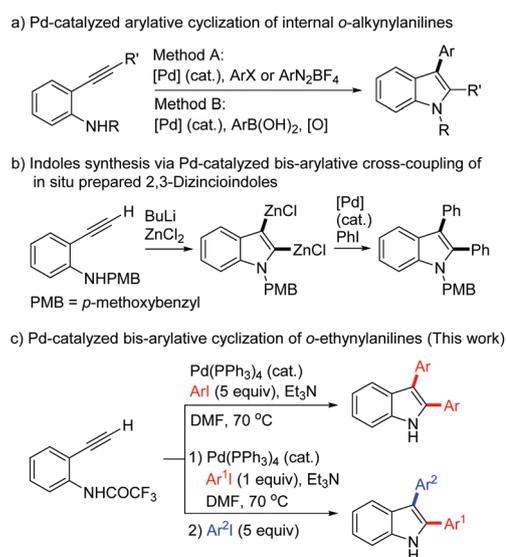
**Scheme 1** Synthesis of 2,3-disubstituted indoles via the Pd-catalyzed transformation of *o*-ethynylanilines.
