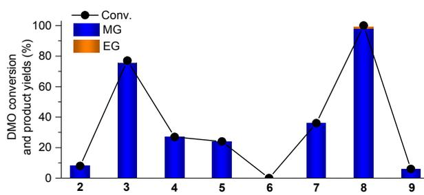
**Fig. 2** Catalytic performance of complexes **2-9** for hydrogenation of DMO into MG (and/or EG). Reaction condition: 11.35 mmol DMO, 0.05 mol% ruthenium, 0.5 mol% NaOMe, 10 mL THF, 50 bar H<sub>2</sub>, 100 °C, 1 h. The conversion of DMO and yield of alcohols were analyzed by gas chromatograph (GC) using *p*-xylene as an internal standard.
