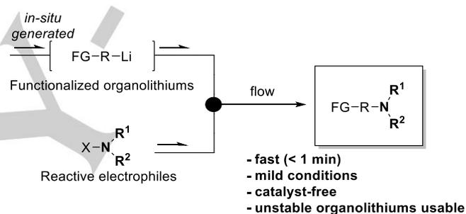
**Scheme 1.** Concept of this work: electrophilic amination of functionalized organolithiums using flow microreactors
