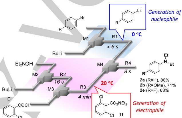
**Figure 2.** Three-step-integrated electrophilic aminations including generation of an aryllithium intermediate, preparation of an aminating reagent, and electrophilic amination.
