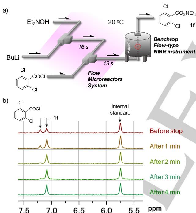
**Figure 1.** Integrated flow system for sequential reactions. a) A flow system including microreactors and a benchtop flow-type NMR instrument. b) Results from <sup>1</sup>H NMR spectroscopy which were detected after 1 min, 2 min, 3 min, and 4 min as well as before stop.
