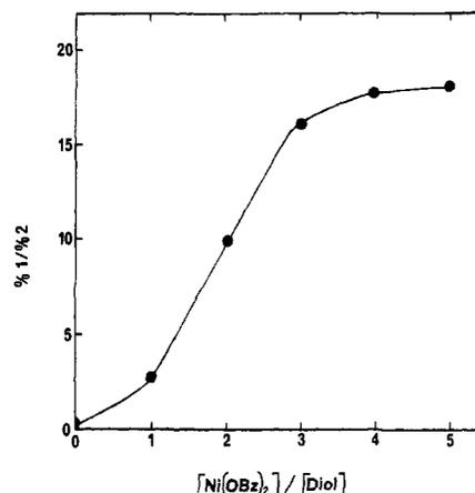
Figure 1. Dependence of selectivity for lactone formation (% 1/2) on the molar ratio of nickel(II) benzoate to 2-ethyl-2-methyl-1,4-butanediol. Reactions were performed at 20 °C in acetonitrile at a constant [Br<sub>2</sub>]/[Ni(OBz)<sub>2</sub>] of 1.6.
