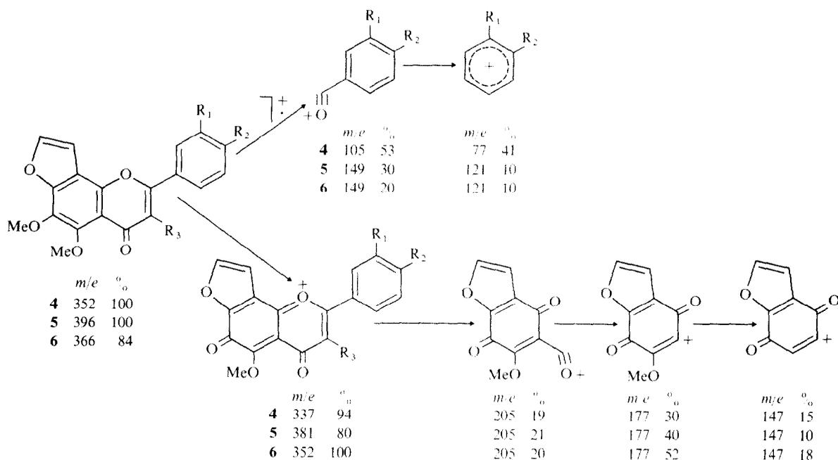
Scheme 2. Principal mass spectral fragmentations of flavones and methylated flavonols **4**, **5** and **6**.
