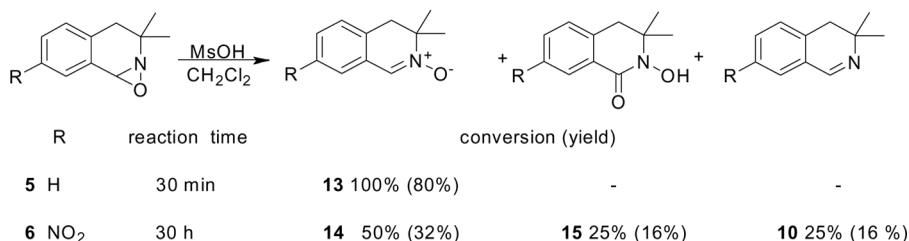
Scheme 4. Oxaziridines **5** and **6** under the action of methanesulfonic acid.
