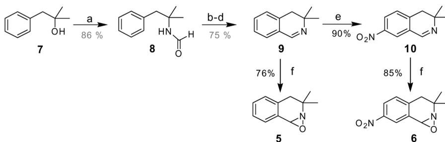
Scheme 2. Reagents and conditions : (a) KCN; SO<sub>4</sub>H<sub>2</sub>-AcOH; rt; (b) oxalyl chlorid; CH<sub>2</sub>Cl<sub>2</sub>; (c) FeCl<sub>3</sub>; (d) MeOH; H<sub>2</sub>SO<sub>4</sub>; (e) KNO<sub>3</sub>-H<sub>2</sub>SO<sub>4</sub>; rt 2 h, 60 °C 4 h; (f) m-CPBA; MeOH.
